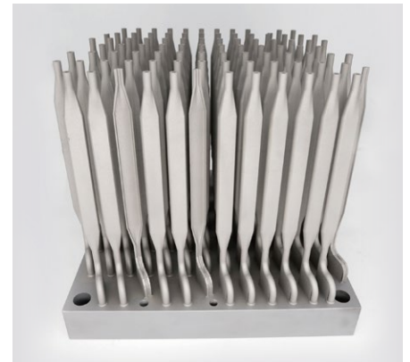
Batch production of industrial pipes printed with stainless steel
