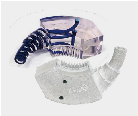
3D printed mold with conforming cooling channels printed with maraging steel
